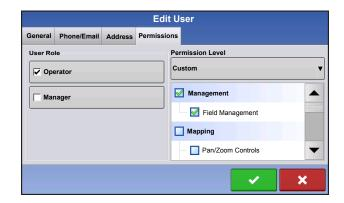
Display uses Traditional mode when Field Management is checked. Events using the Traditional mode are tied to the Grower/Farm/Field structure.
