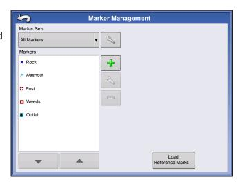
• When creating or editing a marker, check the **Georeferenced Note** button if you wish to add a Field Note that is referenced to the current GPS position when that marker is used.
