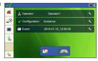
**Operator button** - Allows user to select a machine operator from the drop-down list. Machine operator
