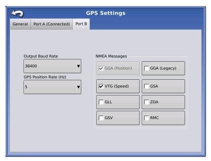
The appearance of this TSIP receiver GPS Port Setup screen is the same for both Ports A and B.
