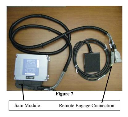
Note: If the installation requires a longer cable PN: 4002140 Remote Engage Extension Cable may be needed.
