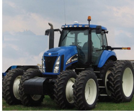
Figure 5-5. Machine ballasted with full set of front suitcase weights and rear wheel weights. Wide stance with duals front and rear for stability and traction.
