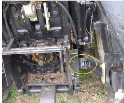
Figure 5-6. Vehicle 3-point sway block set tight and spaced evenly on both sides.
