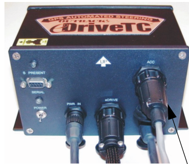
Steering wheel switch cable (refer to the steering wheel kit instructions (part number 876-0082) to install the steering switch cable)
