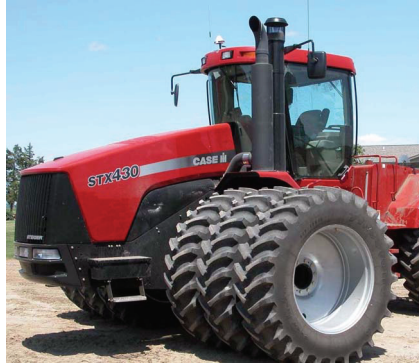
Figure 5-2. GPS antenna installed on the leading edge of the vehicle cab and centered left to right.
