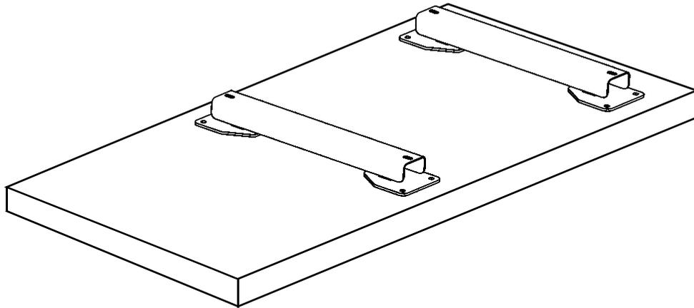
2. Ensure that the load bar feet sit flat on the board or concrete pad.
