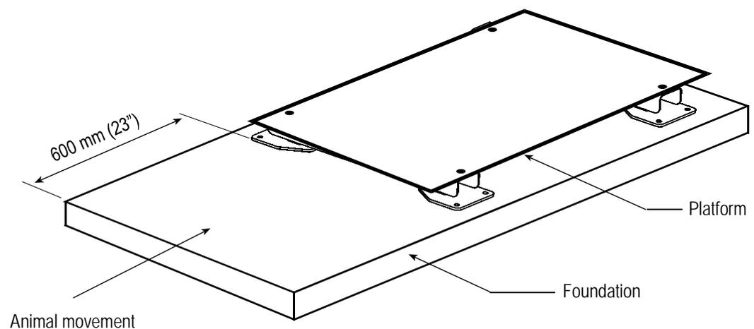
Mounting the load bars on an uneven surface or failing to adequately secure the platform may result in weighing errors.
